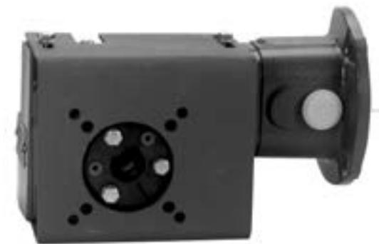
The Output Flange Kit is used to mount the reducer to a flat surface perpendicular to the output shaft. Each kit consists of a fabricated steel flange and required mounting hardware. Specify B-side or H-side mount.
