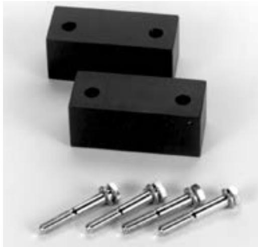
Riser blocks allow clearance over the motor eliminating the need to invert the reducer (worm under) when the application calls for a "ceiling" mount such as under a conveyor or other equipment. Riser blocks permit the reducer to be mounted in the most desirable position keeping the high speed shaft seal above the oil level. Experience shows that this results in increased seal life and durability. Each kit includes the riser block and required mounting hardware.
