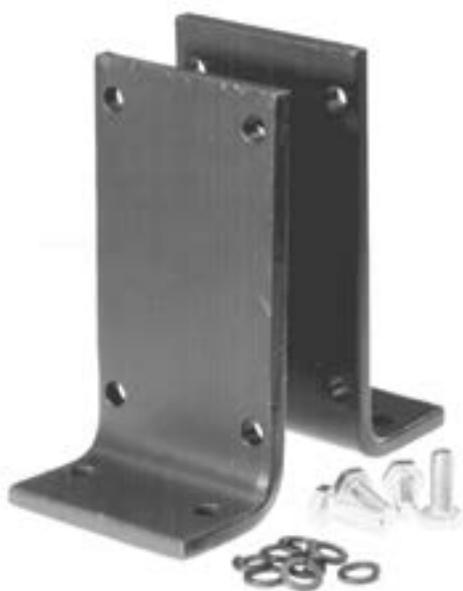
J-mount kits allow the reducer to be "floor" mounted with the motor in a vertical (up) position. In this configuration, the output shaft(s) is horizontal. Each kit includes two brackets and the required mounting hardware.
