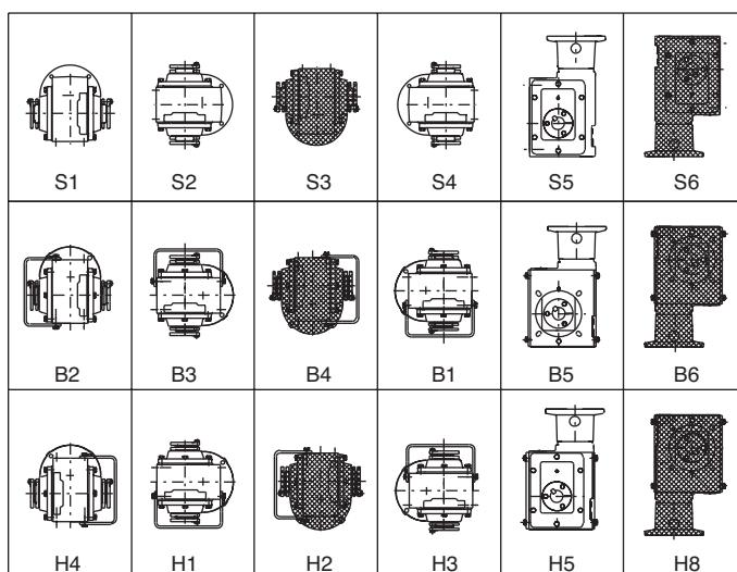
Mounting Positions - Solid Output Shaft
